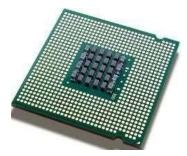
A microprocessor incorporates most or all of the functions of a central processing unit (CPU) on a single integrated circuit (IC).
